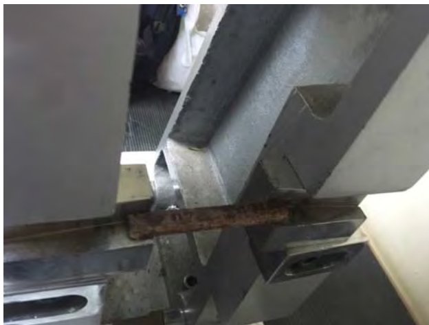
Figure 3.26: XJJU-5.5/50J Izod & Charpy Impact Tester
