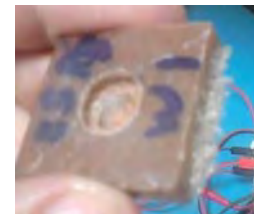
Figure 4.12: Typical Wear Sample
